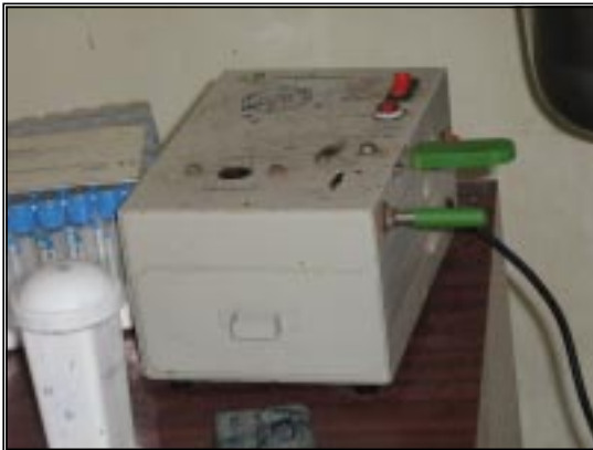
Electrical needle destroyer used for mutilation/destruction of used disposable syringes
