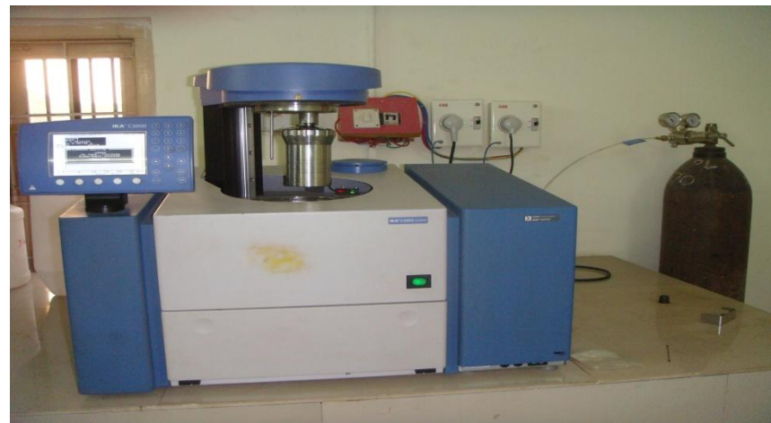
IKA Bomb Calorimeter for testing Calorific Value
